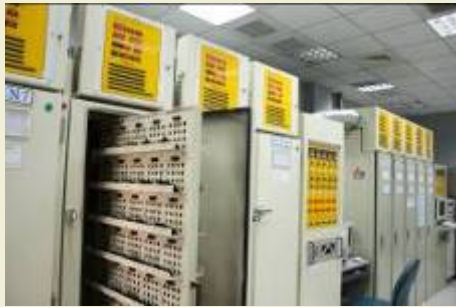
Burn-in Test Instrument for MTTF
